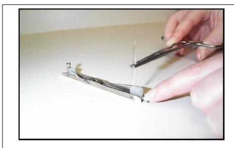
The leading edge of the rod must be oriented in the same direction as the leading edge of the retracting head. In this photograph both are marked with liquid paper. Be careful not to brush the leading edge of the rod against fingers or forceps as this will disturb the silicone coating.
