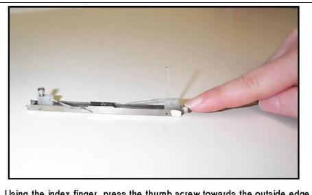
Using the index finger, press the thumb screw towards the outside edge of the retracting head. The square opening of the block should now be facing upwards. This is the point of insertion for the rods. See photograph below.
