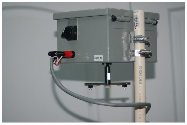
Since the GRIPST 2009 is a non-selective sampler it will collect all air-borne particles, including debris. This should be an important consideration when setting the timer. For continuous operation, we suggest collection cycles of one minute in every ten, or a 10% duty cycle, so that the samples are not overloaded.
